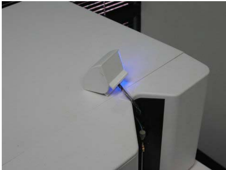
3. Tape LED mechanism out of your way
