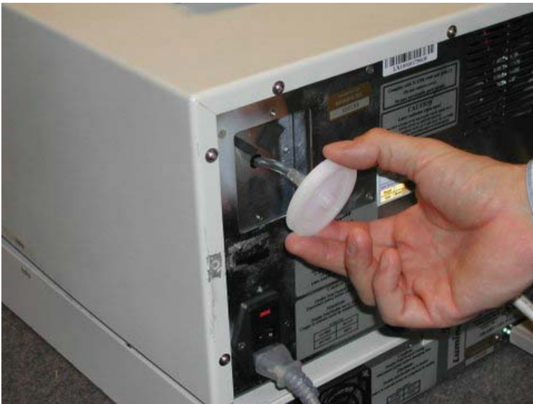
3. Gently pull filter out to remove
