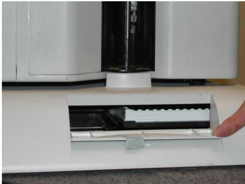
6. Retract plate while holding door open and tape in place
