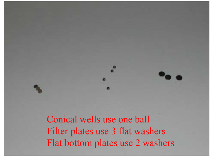
5. Insert plate with proper spacers at the bottom of well A1
